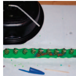
Figure R: The first row of magnets about to go in (epoxy has already been applied, magnets are stacked in the lower left)
