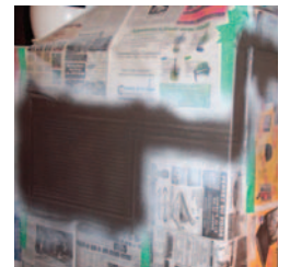
Figure G: Our first coat of conductive paint. Keep adding more coats until the can is empty, or nearly empty if you want to keep a bit "just in case."
