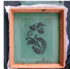
Figure J: Hold the image flat with a piece of glass and expose it to UV light. Watch out for shadows!
