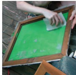
Figure G: Mix emulsion and spread it onto the screens
