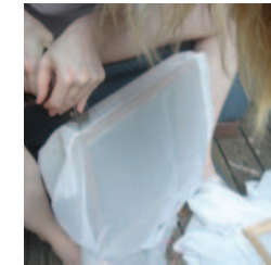
Figure E: Staple the fabric along the edge of the frame, stretching it as you go, and keeping the grain straight
