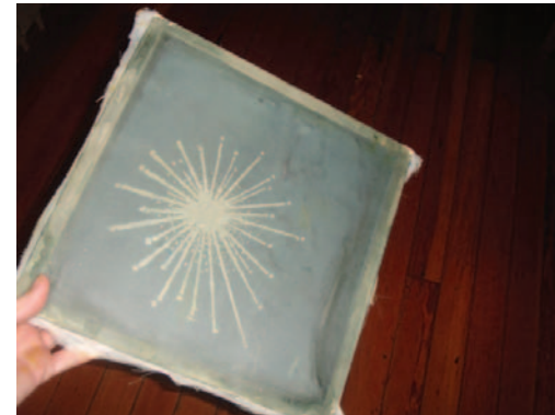
Figure K: Rinse the screen carefully
