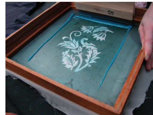
Figure M: Spread some printing ink along the top of the screen and squeegee it over the the image
