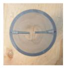
This is the spark gap that will ignite the fuel, firing the cannon.
