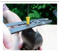
4d. Cover the stun gun test leads (inboard electrodes) with wire nuts cut down to size, or other high-voltage insulators. Insulate all exposed metal areas of the ignition path on the stun gun and bolt electrodes, with electrical tape or silicone glue. It's easy for electricity to find its way underneath any insulation gap at the base of the electrodes
