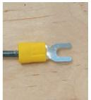
4c. Attach ignition wires to stun gun electrodes by crimping on the modified butt connectors.
