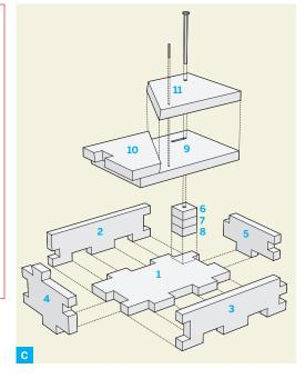
in piece 9 that your screw will slide through (to cut the slot, drill each end and then thread in a saw blade). Also drill smaller holes in the pieces for the locking pin, running the drill only partway through piece 9. Drill both holes with the 2 pieces stacked together to make sure they align.
