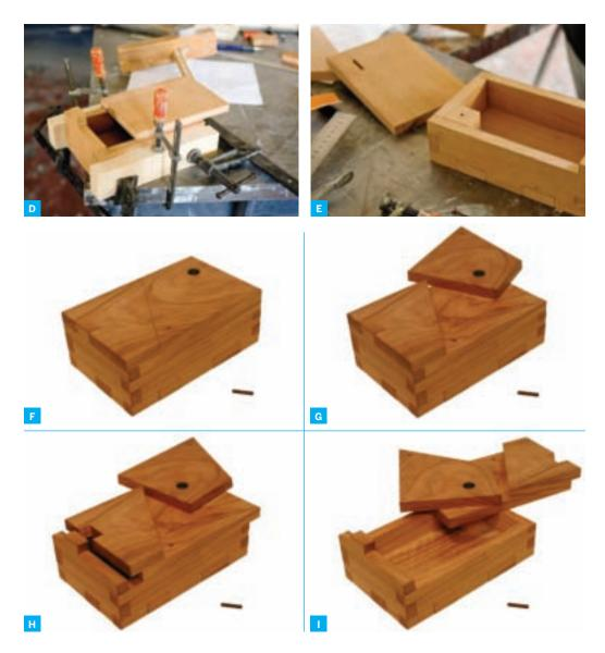
drill pieces 6-8 to hold the bottom of the pivot screw (Figure E).
