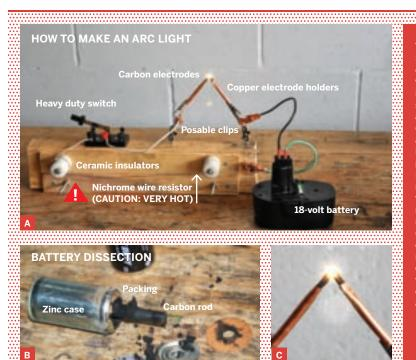
THE DAZZLING SPLENDOR: You can build Sir Davy's world-changing 1807 invention out of simple materials such as copper and carbon (Figure A), powered by a 12V or 18V battery instead of Davy's primitive voltaic cells. He used charcoal, but nowadays it's easiest to get your carbon rods straight out of non-alkaline batteries (Figure B). When electricity is applied, small bits of hot carbon jump across the gap, producing a dazzling incandescent arc (Figure C).
