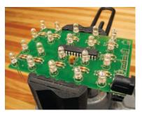
1f. Turn the board upside down on a hard, flat surface to ensure all LEDs are lined up. Solder, and clip the leads. Remove any spacers using hemostats or fine pliers. Notice that the common rail is connecting all the positive (+) pins of the LEDs. (In some other LED projects there is a common ground (-) for all the LEDs.)
