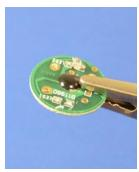
d. Solder one end of the stranded wire onto one of the solder points. Repeat for the other 3. The wires soldered near the markings "LED1" and "LED2" on the board will be the negative wires, and the other 2 will be the positive. Using a black marker, mark the negative wires.
