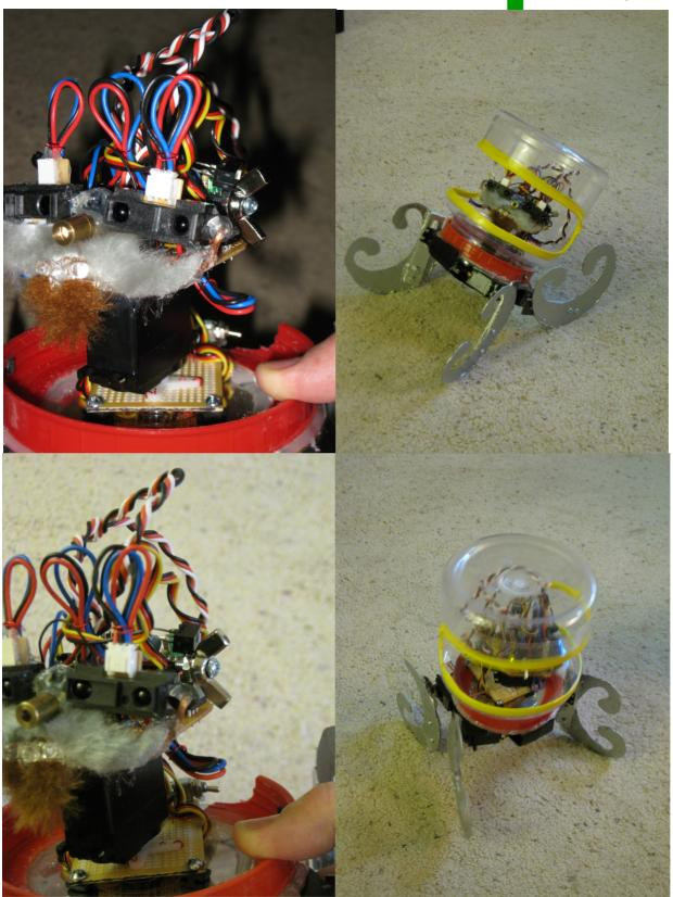
The red jar lid was cut out bolted and glued to the body base CD.
