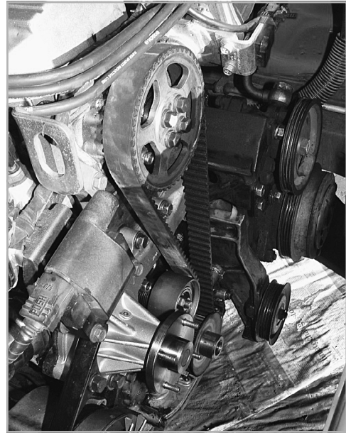
FIGURE 1-10 Timing belt on the engine of a car as a closed pulley system
