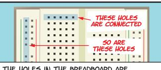
THE HOLES IN THE BREADBOARD ARE CONNECTED IN PATTERNS THAT ALLOW YOU TO ATTACH COMPONENTS TO EACH OTHER AND TO POWER AND GROUND.
