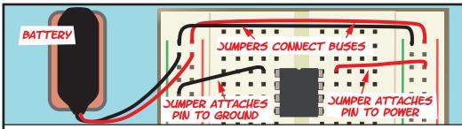
YOU CAN MAKE CONNECTIONS BETWEEN ROWS OF TIE-POINTS BY INSERTING SHORT PIECES OF WIRE CALLED JUMPERS BETWEEN HOLES IN DIFFERENT ROWS.
