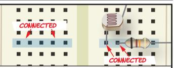
HERE A RESISTOR IS CONNECTED TO POWER AND TO THE ANODE OF AN LED. THE OTHER
