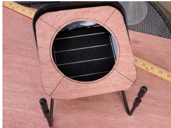
Figure 1-15. Use a coping saw or jigsaw to cut out the large hole in the center and outline of the plywood plate.
