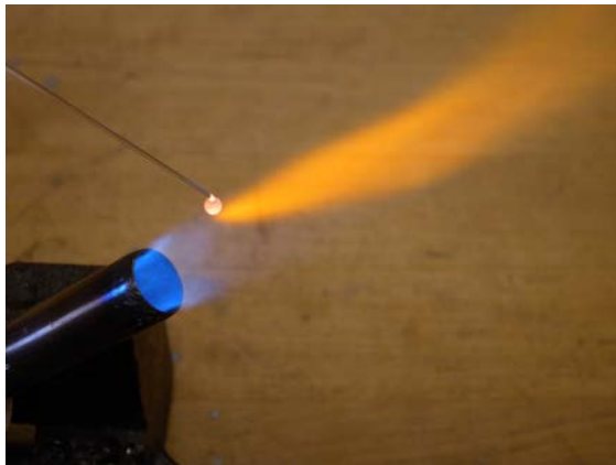
Figure 8-10. Remove the glass from the flame as soon as you create a 3-4mm ball lens. If the lens gets too big, it might fall off of the filament.
