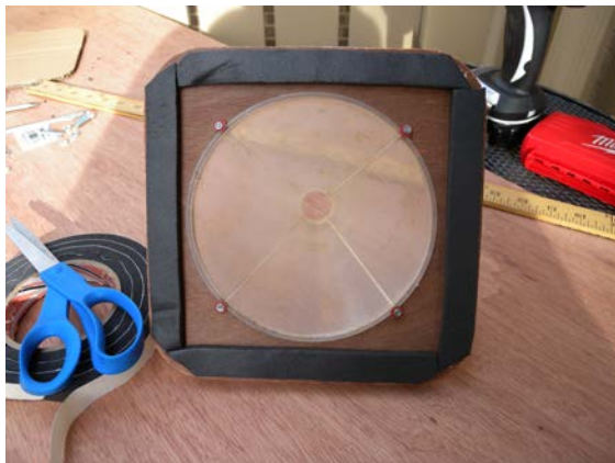
Figure 1-16. Attach foam tape to the back of the plywood plate to prevent any air leaks.
