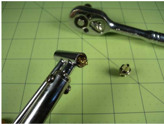
Figure 4-61. Make sure that the brass wool does not clog the air inlet.
