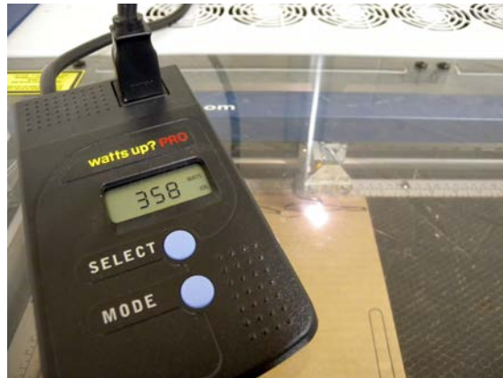
Figure 1-4. Digital Watt meters can accurately display a piece of equipments' power consumption in real time
